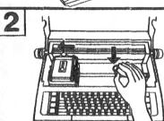
Move carrier to left side of typewriter. Then place yellow plastic on carrier guide rod with one end touching right side of frame.
